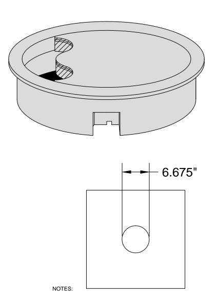
1 RECOMMENDED FLOOR TILE CUT-OUT DIMENSIONS - CENTER OF TILE =  $6\frac{5}{8}$  "
