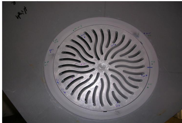
Close-up of Diffuser Under Test (Test Points in Blue)
